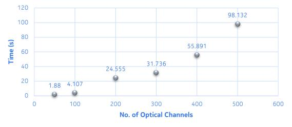
These measurements include the computation time of the optimal optical channel migration sequence.
