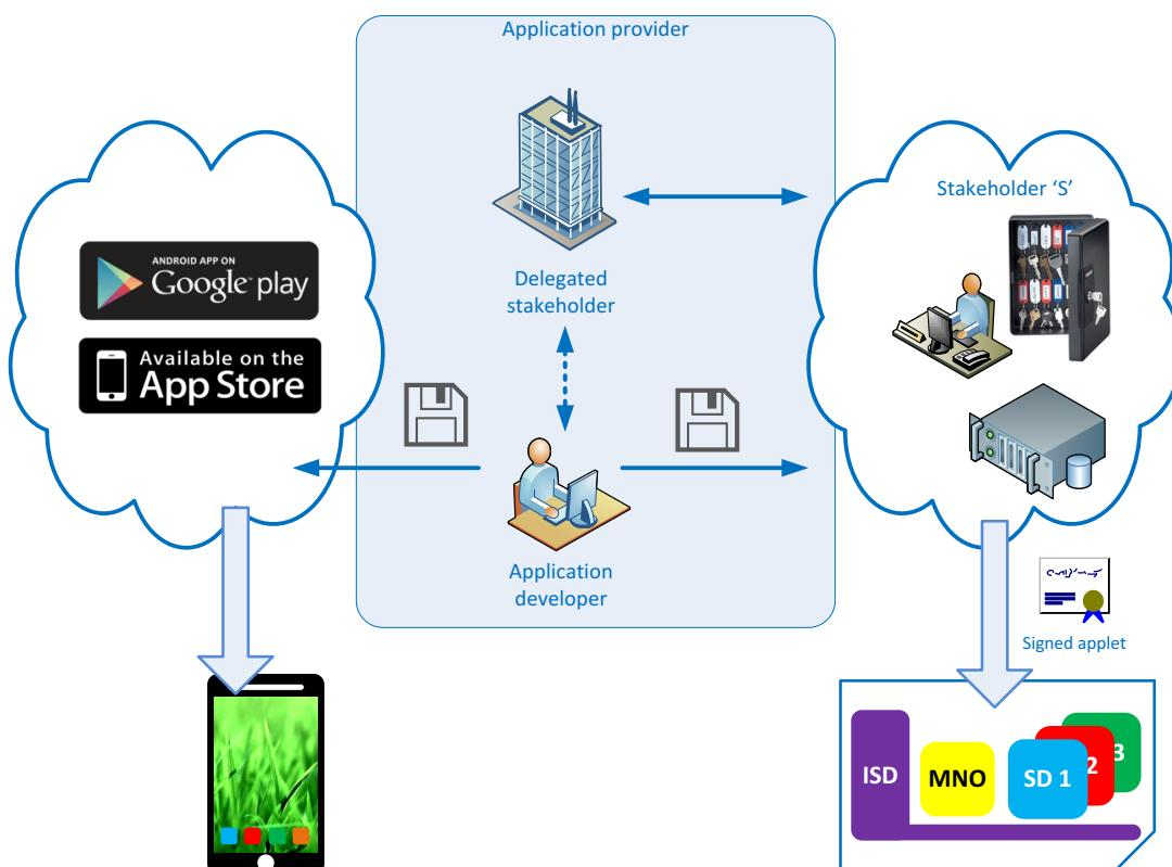
Figure 1 Visualization of the open market code distribution model. ISD= issuer security domain (NREN's domain), MNO = profile of mobile operator, SD = security domain of institution.
